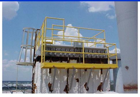
This pulse jet conversion was done turnkey for a Florida cement plant that was having problems meeting their desired conveying rates to their finish silos. CS&S was able to add 50% more capacity to an old shaker unit for less that 45% of the cost of new equipment. We can do the same for your company.
